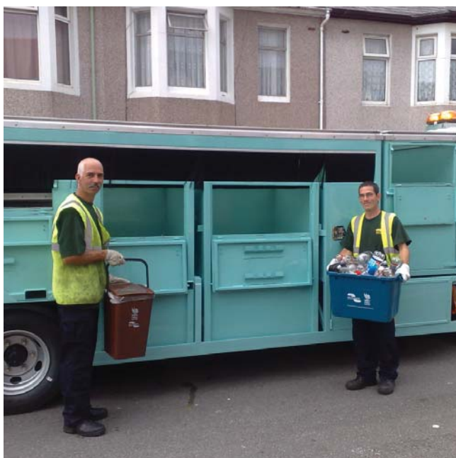
Collection operatives for Newport Wastesavers hand sort recyclable wastes into separate compartments in a kerbside sort collection vehicle.
